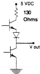
and diode at 11 mA would approximate 0.8 volt; and the drop across 130 Ohms is 1.4 volt. This 2.2 volt drop would leave only about 1.8 volts for the relay to operate, not enough for relay turn-on.
