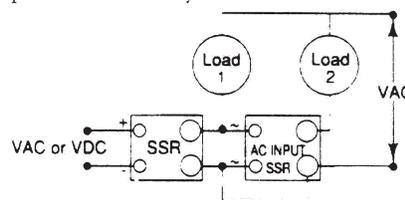
All WRC Solid State Relays with DC input and AC output have a control circuit consisting of 1500 Ohms in series with the Opto-coupler LED. At 3 Volt input the relay will turn on with 1.33 mA (3 volts-1 volt dropped across the LED = 2 Volts / 1500 Ohms = 1.33 mA).
