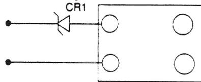
Two SPST AC SSR's controlled from a single DC source, can be connected to operate as a SPDT relay to switch AC power to either of two loads. Note that one of the SSR's must be an AC input type. Because of overlap (make-before break), the power source must be capable of supporting both loads for approximately two cycles. Offstate leakage in load No. 1 will be equal to the off-state leakage of relay No. 1 plus the input current for relay No. 2.
