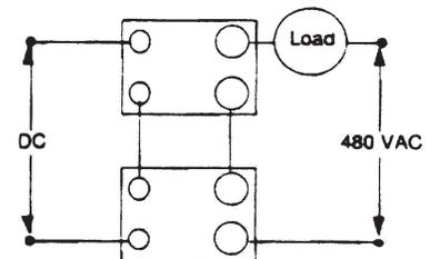
An AC SSR can be made to self latch (at the sacrifice of input-output isolation), thus permitting the use of momentary action switches for on/ off or stop/start operation. It may be necessary to insert an RC filter across the relay input to prevent the relay from turning on due to switching transients upon application of system power. Note that the SSR employed here must be an AC input type.
