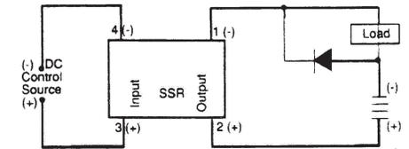
Input and output polarity must be observed. Inductive loads must be diode suppressed.
