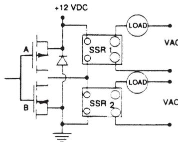
When sourcing transistor A is on, it conducts current to SSR2. When sinking transistor B is on, it conducts to SSR1.
